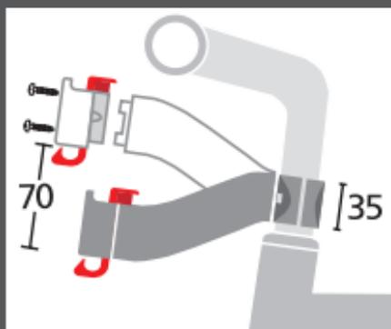
**Handlebaradapter** for mounting on stem. Allows lower accessory position, independent from inclination of adjustable stems. Bracket offers 2 mounting positions in different heights. Before mounting please add rubber stickers in clamp.
